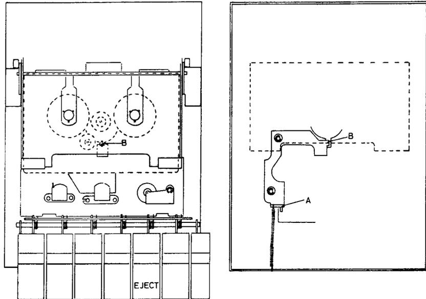
Eject should be adjusted so that notch B locks the cassette holder when the latter is pressed down and so that it releases positively when the Eject button is depressed (with all other buttons released).
