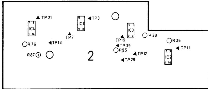
Tune the receiver correctly to an FM station (0 V between pin 5 and pin 6 of 2IC2 (2TP12 and 2TP29).
