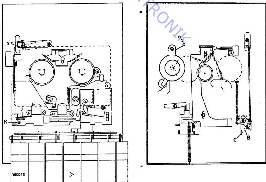
Arm A should be adjusted (bent) so that angle B provides positive locking of arm C (Record button) when a cassette is inserted with the record lock window open and so that arm B is positively disengaged from arm C when the cassette record lock window is closed.
