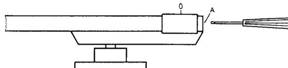
Set the stylus-force adjustment slider to the 0 position. Adjust screw A until the pickup arm is only just in balance. Thereafter set the stylus force to the recommended value.
