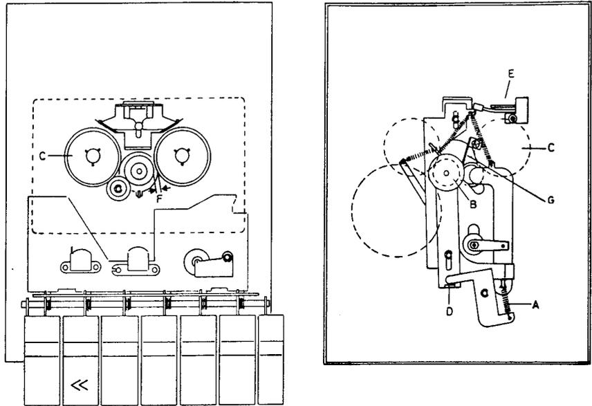
With the unit set at Stop, adjust leaf spring G so that spacing F  $\leq$  0.4 mm. Spring A should be only just tight enough so that the transmission slips in the clutch below idler wheel B when reel C is held fast. It may be necessary to adjust or replace clutch B. Switch E should be ON.
