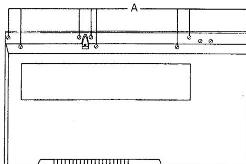
Remove screws A and B.
