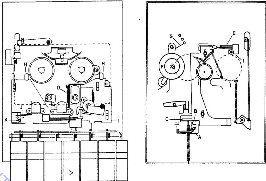
When the Play button is in its depressed and locked position there should be contact between A, B and C; and spring D should be tight. Also, plate I should go all the way forwards against stop blocks H.
