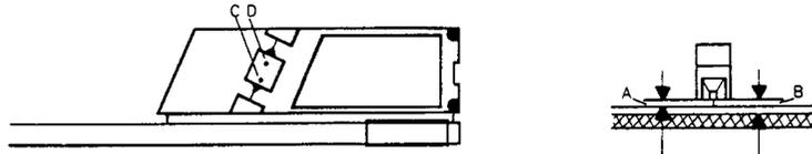
With screws C and D adjust so that distances A and B are identical and the plane portion of the pickup is parallel with the top side of the record. Adjustment is performed with a counterbalance weight inserted.
