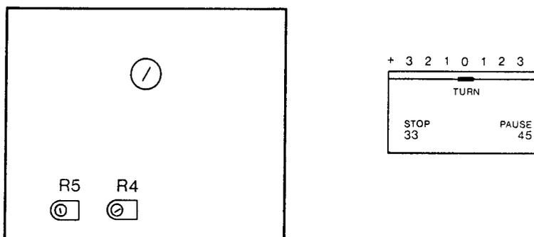
Set the scale for speed adjustment to 0.
